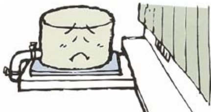
Vibration is more easily transmitted to the building.
